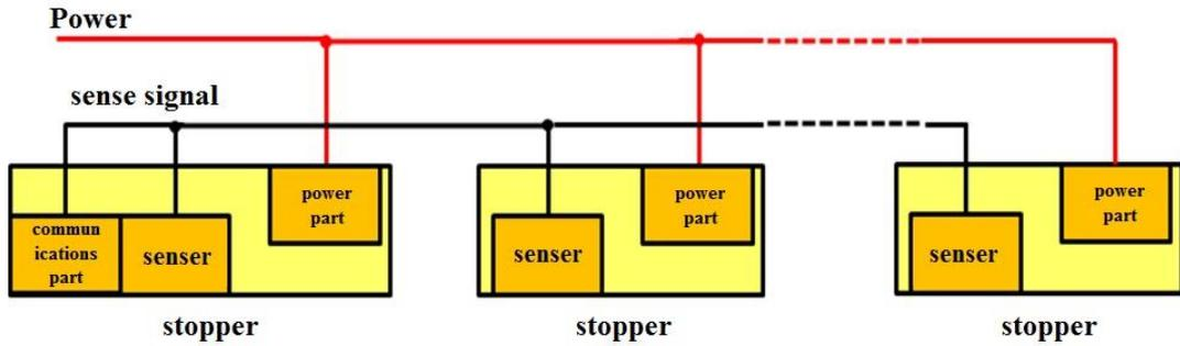
Figure 7. Wired connection method between sensor embedded stoppers
