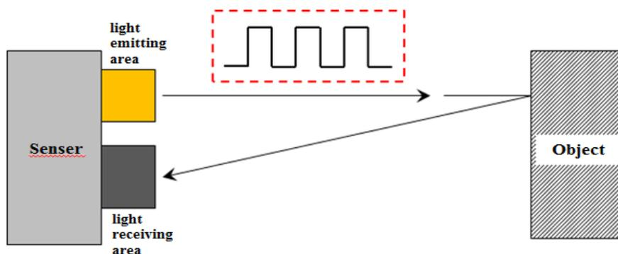
Figure 4. Light-emitting and receiving method of the optical sensor
