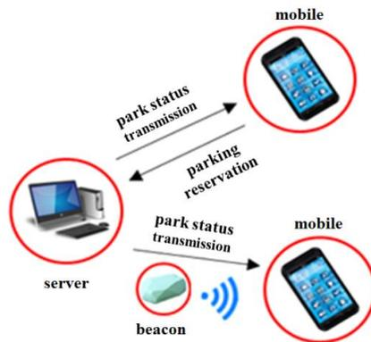
Figure 8. A flowchart about how to transmit parking status information
