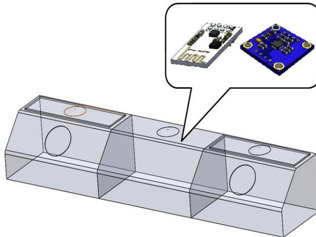
Figure 5. Parking stopper internally equipped with a detecting sensor
